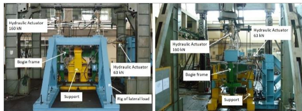
Figure 5. Monorail frame bogie prototype static test setup
