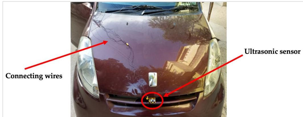
Figure 7. Ultrasonic sensor at the front of the vehicle to calculate the actual braking time
