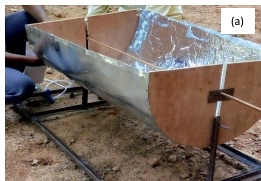
Figure 3. (a) Fabrication of Solar Parabolic Trough Collector; (b) View of Condenser, Cold storage box and Absorber Unit
