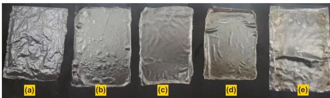
Figure 1. Product of CMC film: (a) CMC-control; (b) CMC-glycerol 0.5%v/v; (c) CMC-glycerol 1.0%v/v; (d) CMC-glycerol 1.5%v/v; (e) CMC-glycerol 2.5%v/v
