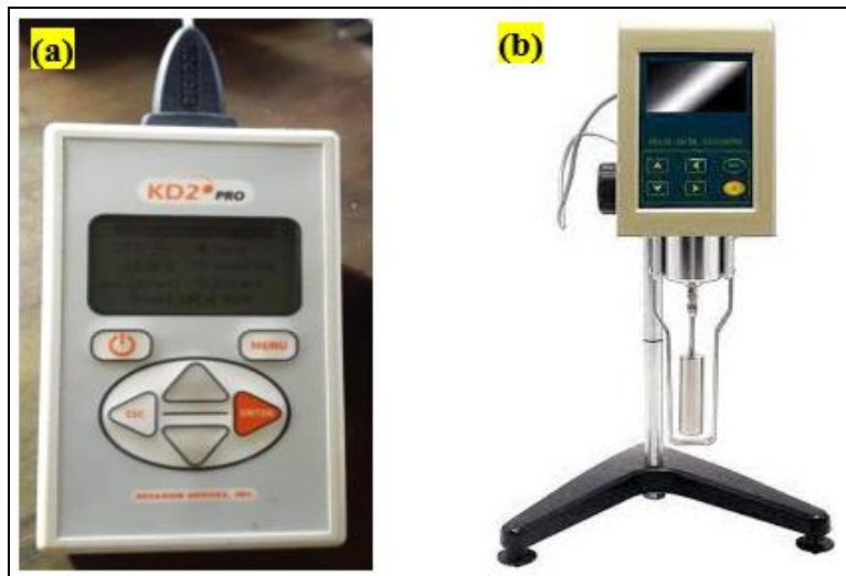
Figure 2. Thermophysical properties testing equipment: (a) Analyzer KD2 Pro; (b) NDJ-8S Viscometer
