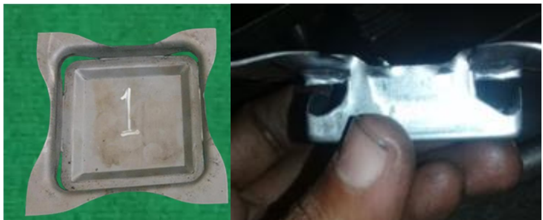
Figure 2. Instances of tear defects observed during the execution of square cup deep drawing
