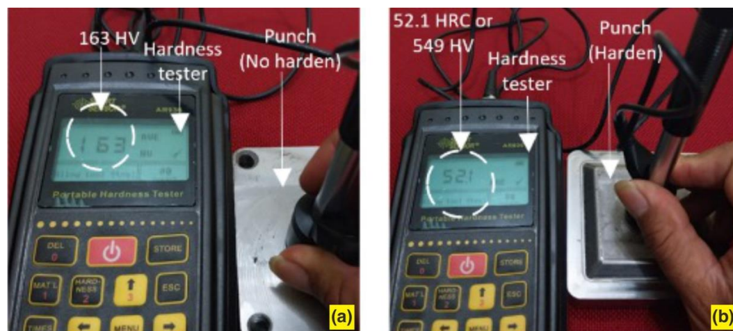
Figure 7. Alloy steel SKD 11: (a) No hardening process, (b) After-hardening process
