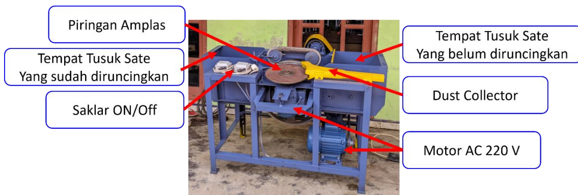
Gambar 4. Mesin peruncing tusuk sate
