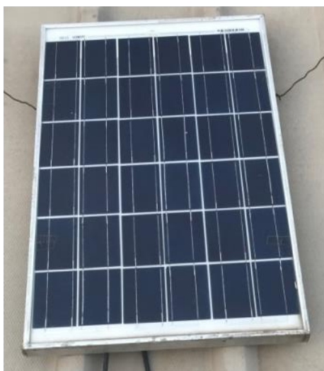
Figure 3. Front view of the 10W solar panel used.
