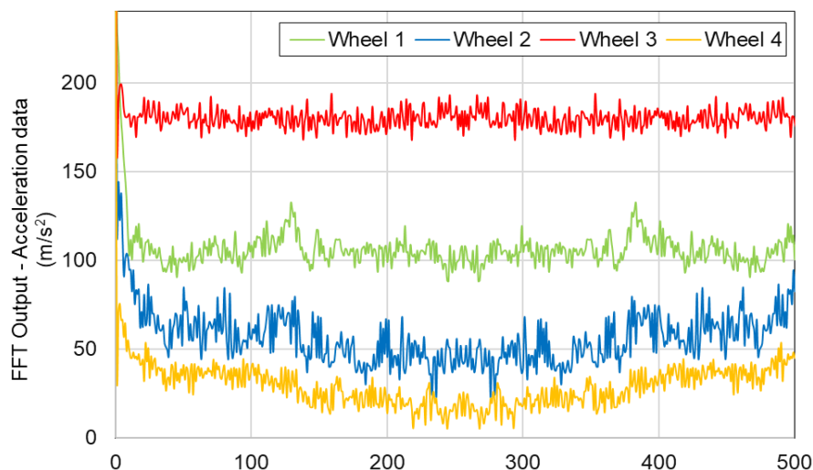
Figure 9. Acceleration data as output of FFT process
