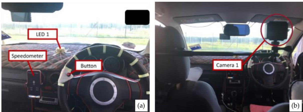
Figure 4. The Interior of the instrumented car: (a) location of LED 1, speedometer, and button, (b) location of the Camera 1
