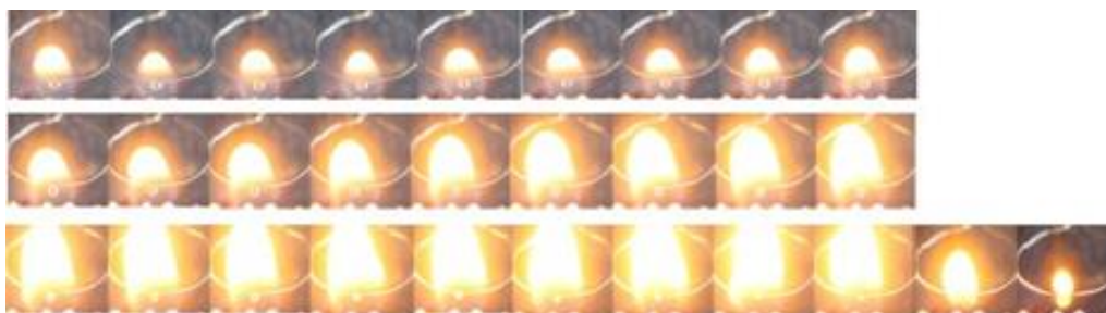
Figure 8. Flame evolution of CCO droplet
