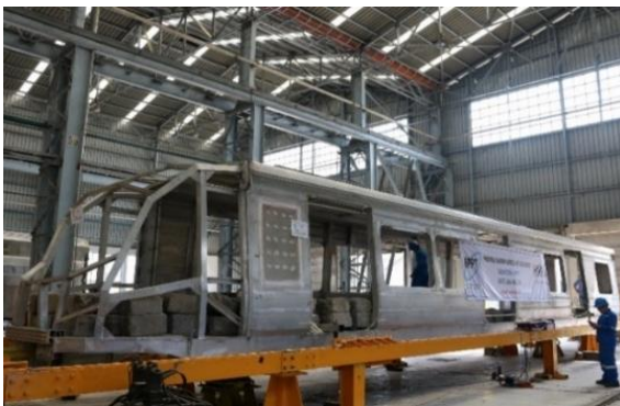
Figure 3. LRT cabin train as a test specimen
