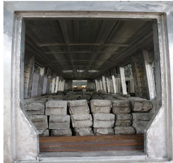
Figure 4. Vertical load test using bataton
