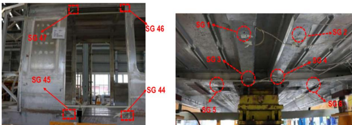
Figure 7. Example of a strain gauges installation location
