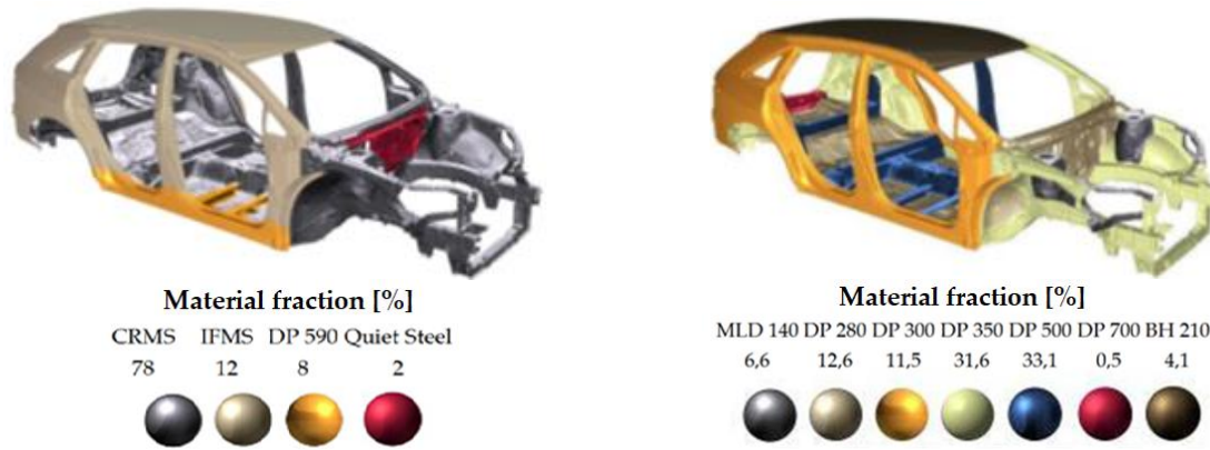
Figure 10. Weight Fraction of Materials in BIW for Baseline (left) and Low Development (right)
