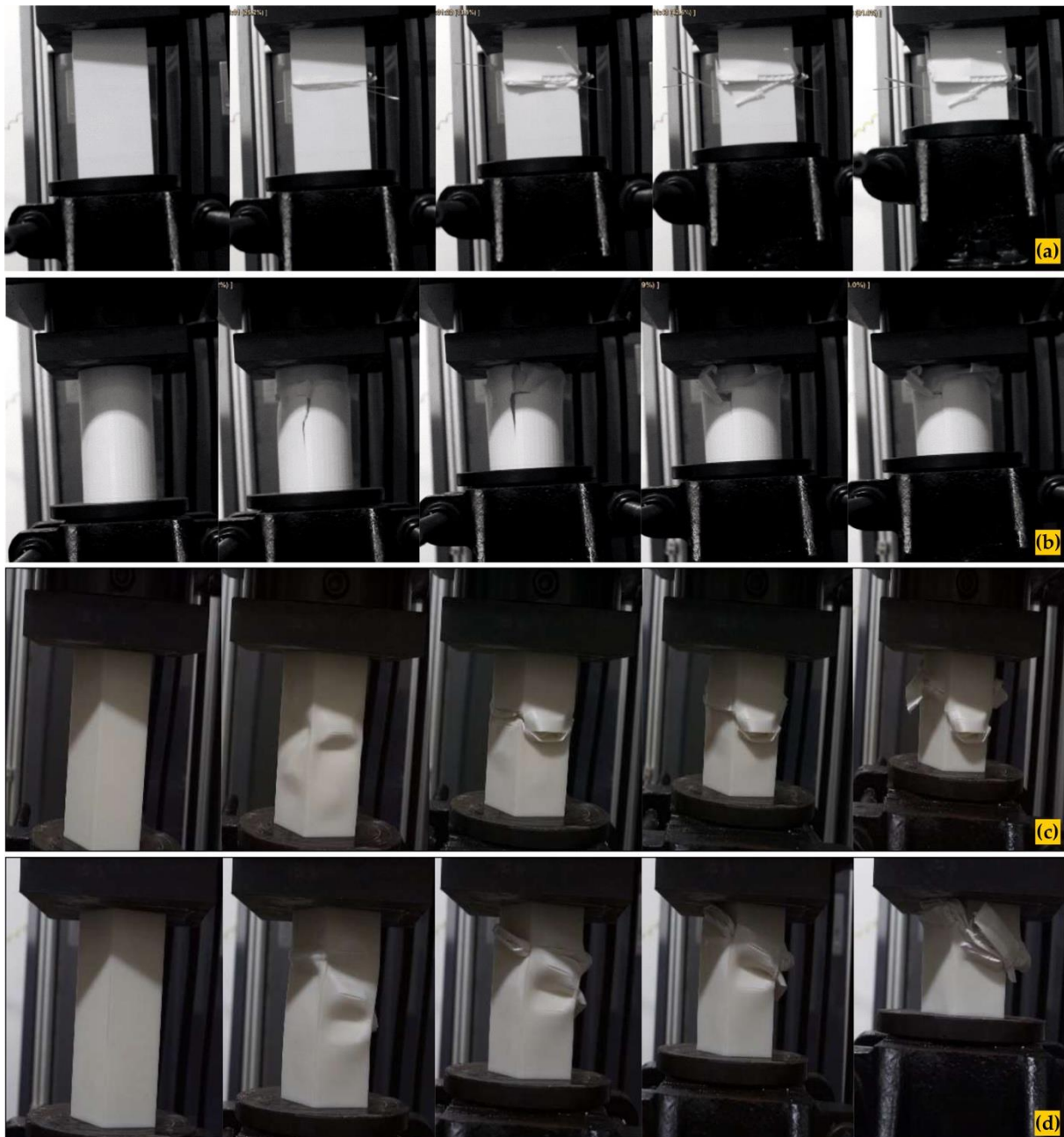
Figure 7. Collapsed specimens (a) Multi-cell square (MCS) (b) Multi-cell circle (MCC) (c) Multi-cell pentagonal (MCP) (d) Multi-cell pentagonal circle (MCPC)
