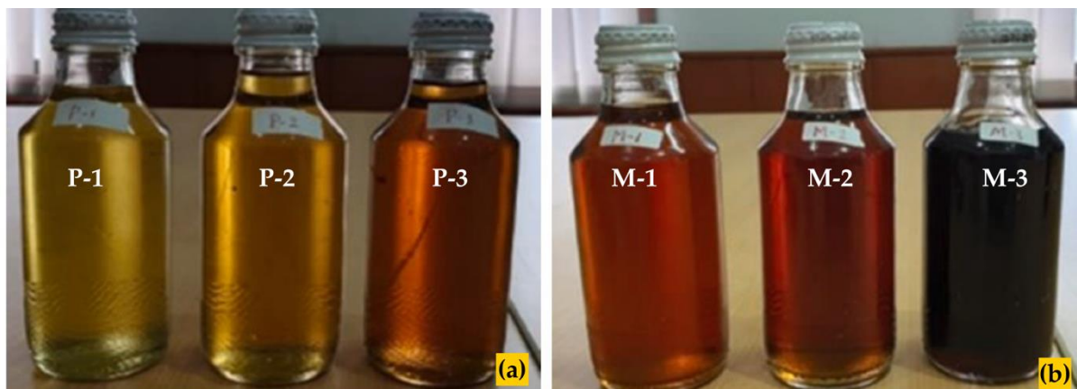
Figure 4. The difference in PPO color obtained depends on the pyrolysis temperature of: (a) LDPE Plastic-P; (b) LDPE Plastic-M [128]
